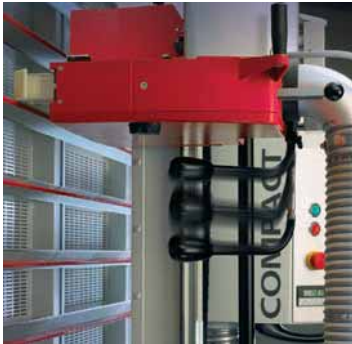
Saw unit with powerful motor (3.9 kW) and length-adjustable operating lever, which significantly facilitates penetration.
