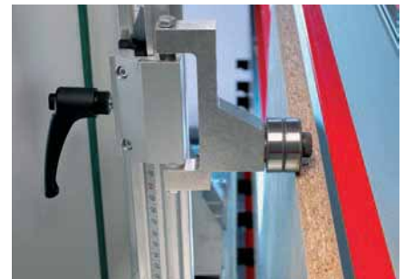
Strip cutting gauge, 400 and 600 mm in length with edge-protecting roller support.
